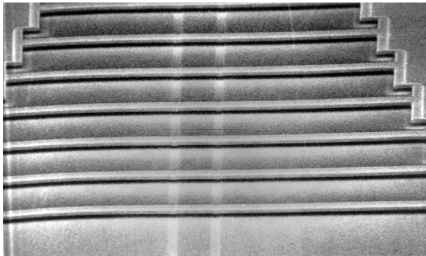
Figure 3.12 SEM of a set of clamped-clamped diagnostic bridges, each beam is 10\text{ }\mu\text{m} wide and 2\text{ }\mu\text{m} thick, with the length varying from 100\text{ }\mu\text{m} to 300\text{ }\mu\text{m} .
